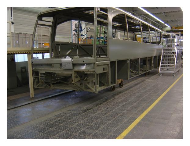
Assembly and finishing of busses up to the final assembly on heavy three-wheeled assembling trestles with steel tyres. Wheel radius 160 mm, width of wheel rim approx. 60 mm.
