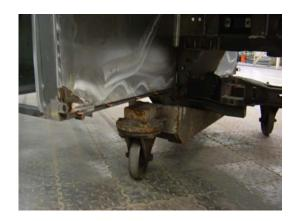
Heavy load on narrow footprints of steelwheels with individual axles. Due to the interlocking panels the joint is minimized, thereby reducing the rolling resistance.
